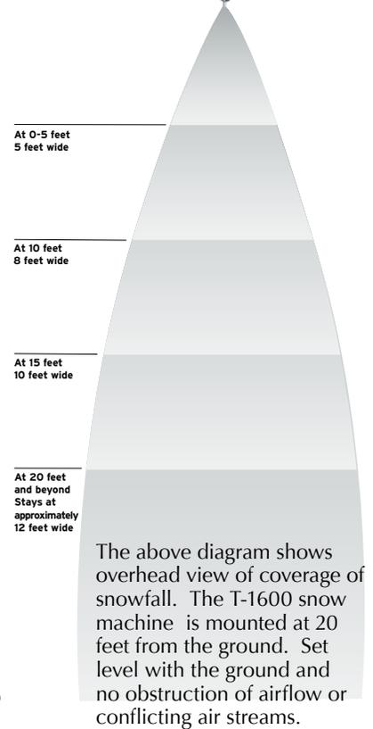
The above diagram shows overhead view of coverage of snowfall. The T-1600 snow machine is mounted at 20 feet from the ground. Set level with the ground and no obstruction of airflow or conflicting air streams.
